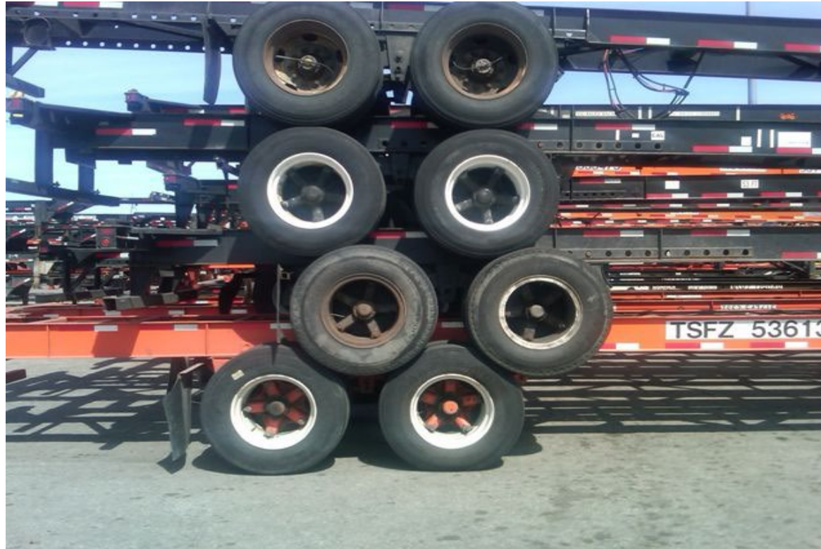
Incorrect Stacking/Tire on Tire
